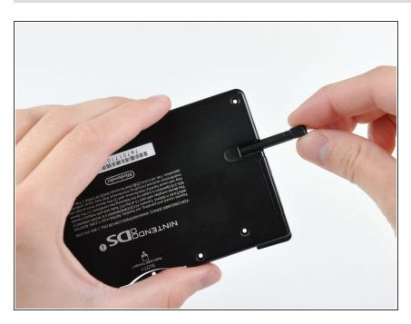
Pull the stylus straight out its housing and remove it from the rear case.
