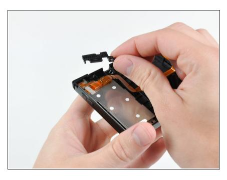
Lift the right trigger button cover out of the rear case.
