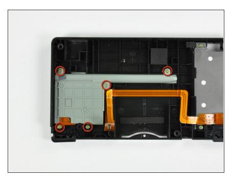
Remove the five 3.9 mm Phillips screws securing the stylus holder to the rear case.
