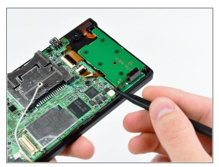
Use the tip of a spudger to pry the power board connector out of its socket on the motherboard.
