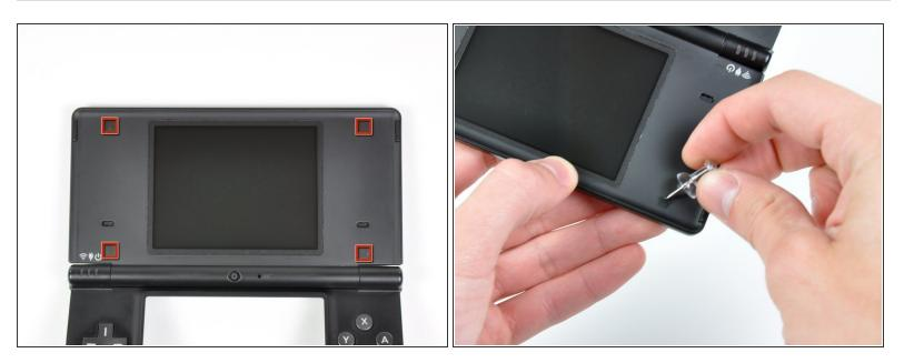
• Use a pushpin to remove the four plastic screw covers (highlighted in red) on the front bezel.
