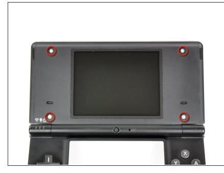
Remove the four Phillips screws securing the rear bezel to the front bezel.
