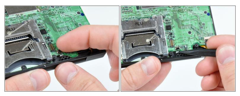
• Use your fingernail or the edge of a plastic opening tool to carefully flip up the touchscreen ribbon cable retaining flap.
