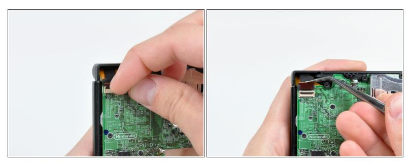
• Use your fingernail or the edge of a plastic opening tool to carefully flip up the dual camera ribbon cable retaining flap.
