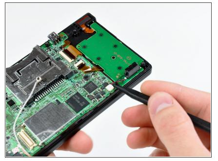
• Use the tip of a spudger to pry the power board connector out of its socket on the motherboard.
