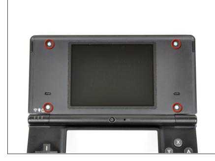
Remove the four Phillips screws securing the rear bezel to the front bezel.
