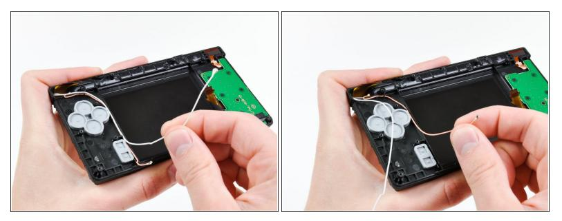
De-route the microphone and Wi-Fi antenna cables through the opening located on the bottom DSi's framework.
