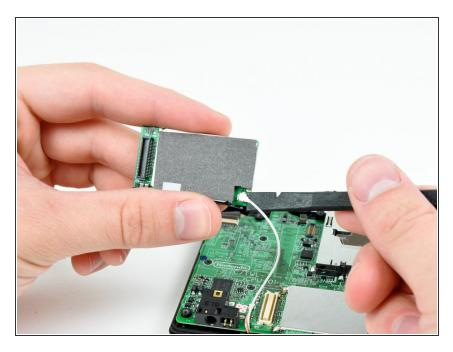
Pry the Wi-Fi antenna connector straight up from its socket on the Wi-Fi board.
