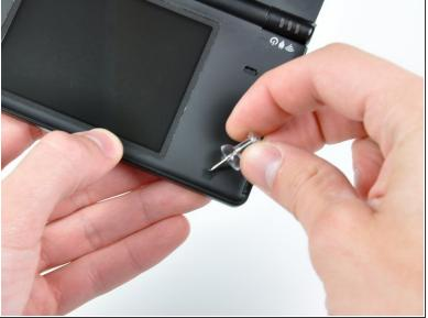
• Use a pushpin to remove the four plastic screw covers (highlighted in red) on the front bezel.
