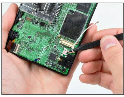
With the tip of a spudger, Pry the microphone antenna up off its socket on the motherboard.
