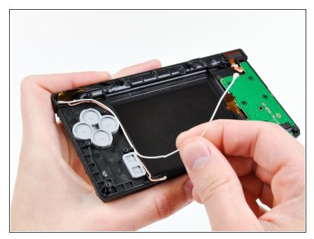
De-route the Wi-Fi antenna cable from its slot in the bottom front bezel.
