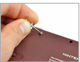
Remove the four rubber screw covers on the lower case by prying them up with a push pin.
