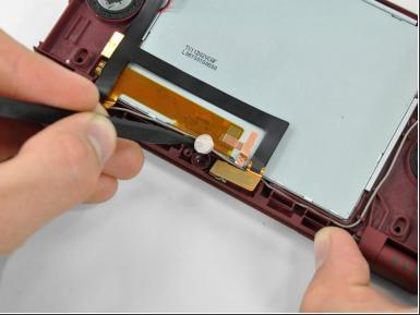
Use the tip of a spudger to lift the microphone from its seat on the front display bezel.
