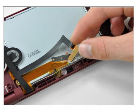
Lift the camera out of its seat on the front bezel.
