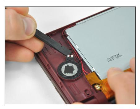
Use a spudger to lift the right speaker from its housing in the front bezel.
