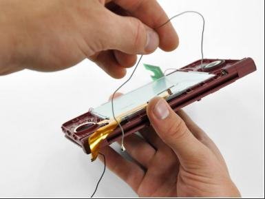
Pull the Wi-Fi antenna cable through the right hinge connecting the front bezel and upper case.
