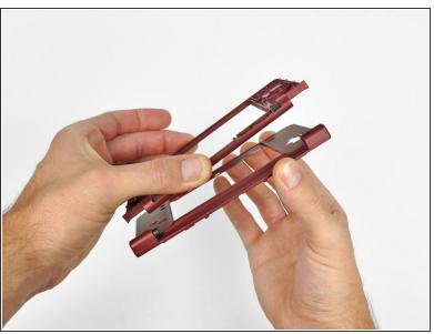
Lift the front bezel off of the upper case, tilting the left side of the front bezel away from the upper case first.
