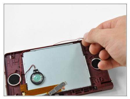
• De-route the speaker wires that run above the upper display screen.
