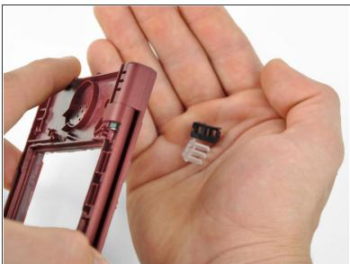
Remove the LED diffuser and black retaining bracket by turning the upper case upside-down and letting both pieces fall into your hand.
