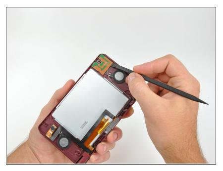
Using the flat end of a spudger, pry the Wi-Fi antenna out of its housing from within the front bezel and move it aside.
