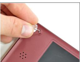
Use a push pin to remove the four plastic screw covers on the front bezel.
