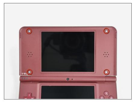
Remove four Phillips screws securing the front bezel to the rear bezel.
