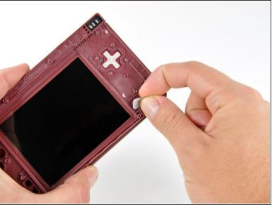
Peel the rubber button pads off the backside of the D-pad and power button.
