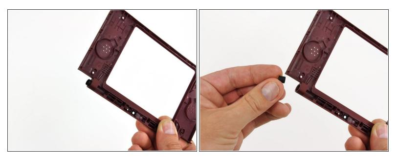
Pull the hollow hinge pin out of the right side of the front bezel.
