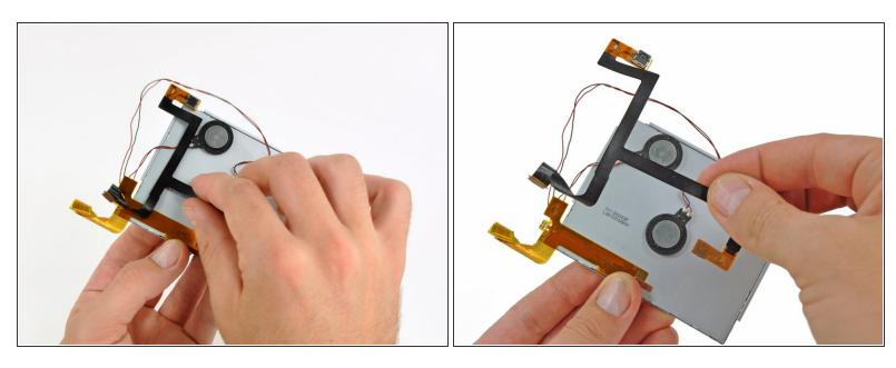
Lift the camera ribbon cable up off the upper LCD, minding any adhesive that may still be attached.
