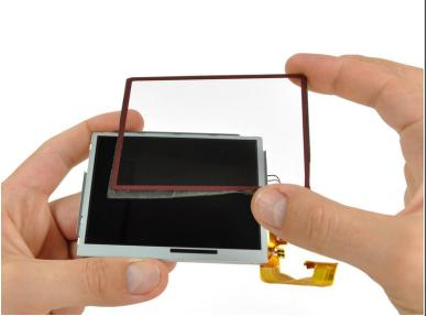
Firmly grasp the upper screen, and lifting from the right edge, pull the upper screen off of the upper LCD.
