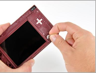
Peel the rubber button pads off the backside of the D-pad and power button.
