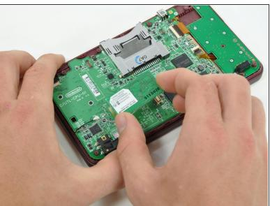
Lift the Wi-Fi board up off its socket on the motherboard.
