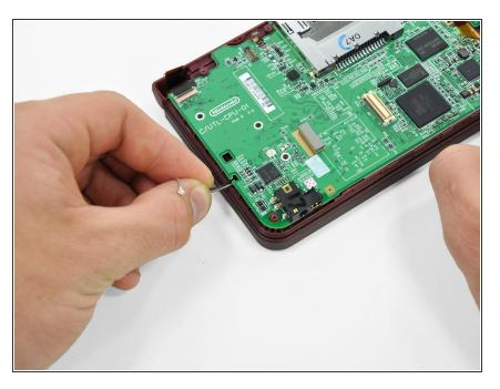
Deroute the microphone and antenna cables through the slot in the motherboard.
