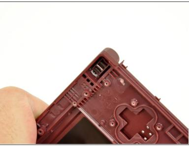
Using a pair of tweezers, remove the LED diffuser bracket and the LED diffuser from the upper case of the DSi XL.
