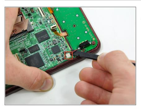
Using the flat end of the spudger, pry the battery cable up off its socket on the motherboard.
