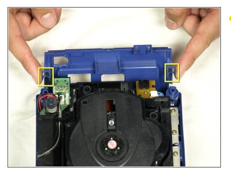
Gently press down on the clips located on either side of the the back panel, as shown, and carefully remove it from the main part of the device.
