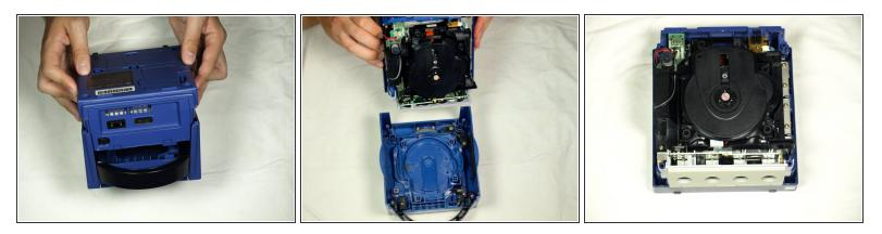
• With the bottom side of the GameCube facing upward and the screws removed, carefully pull the outer shell of the unit away from the top half. Then place the inside of the unit facing up.
