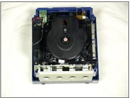
With the bottom side of the GameCube facing upward and the screws removed, carefully pull the outer shell of the unit away from the top half. Then place the inside of the unit facing up.
