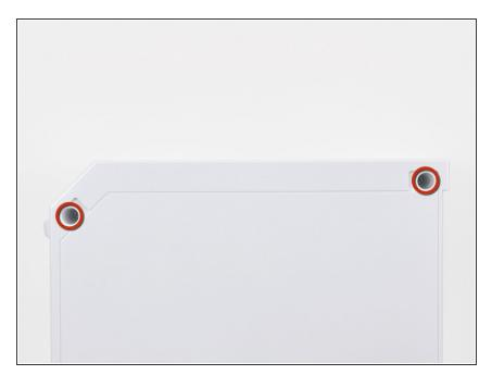
Remove the two 8.2 mm Tri-Wing screws hidden under the feet you just removed.
