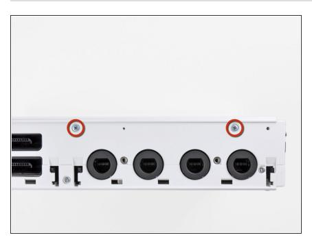
Remove the two 5 mm Phillips screws above the controller ports.
