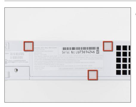
Use a metal spudger to remove the three highlighted screw covers stuck to the side of the Wii.
