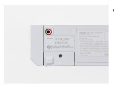
Remove the single 5.9 mm Phillips screw hidden under the foot you just removed.
