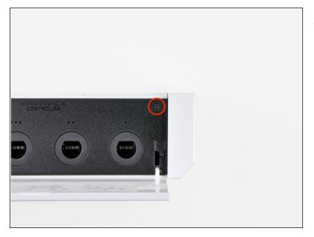
Remove the single 5.9 mm Phillips screw under the controller port door nearest the faceplate.
