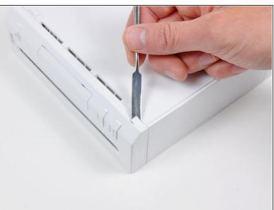
Use a metal spudger to remove the white plastic screw covers stuck to the lower case near the front of the Wii.
