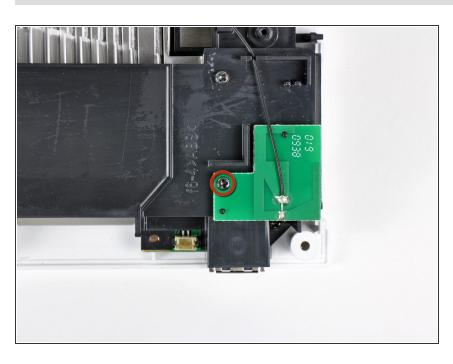
Remove the single 10 mm Phillips screw securing the second Wi-Fi antenna to the top of the fan shroud.
