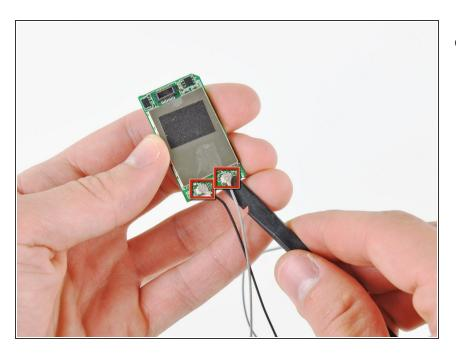
Use the flat end of a spudger to pry both antenna connectors off their sockets on the Wi-Fi board.
