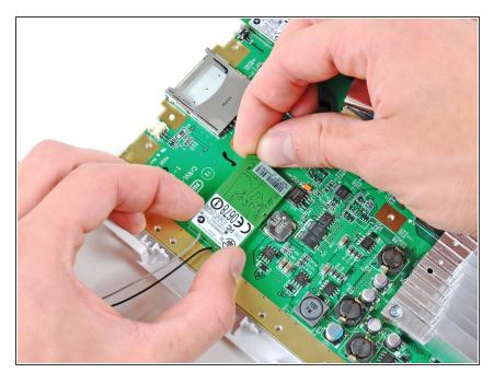
Lift the side of the Wi-Fi board furthest away from the heat sink and lift it out of its socket on the motherboard, being careful not to put too much sideways force on the connector.
