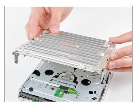
Lift the DVD drive shield upward and remove it from the Wii.
