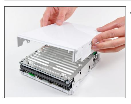
Lift the outer case straight up off the body of the Wii.
