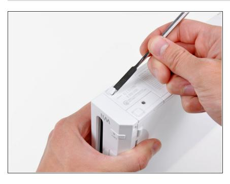
Use a metal spudger to remove the rubber foot stuck to the side of the Wii near the DVD drive opening.
