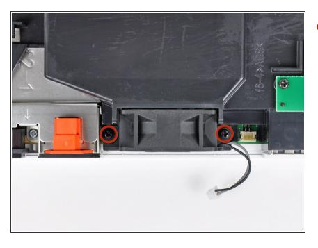
Remove the two 10 mm Phillips screws securing the fan to the fan shroud.
