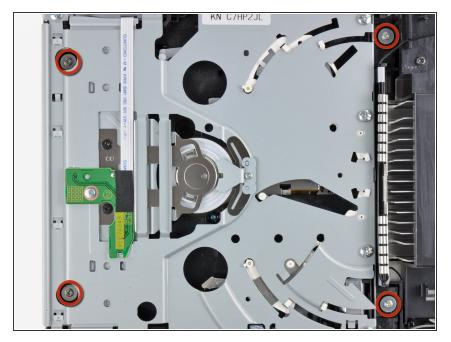
Remove the four 9 mm Phillips screws securing the DVD drive to the bottom panel.
