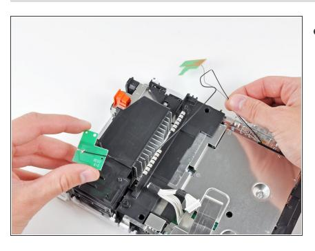
Carefully de-route both antennas from the frame of the Wii and lay them aside.
