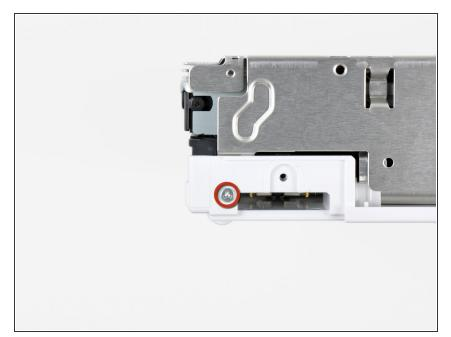
Remove the 8.2 mm Tri-Wing screw that was hidden beneath the battery door.
