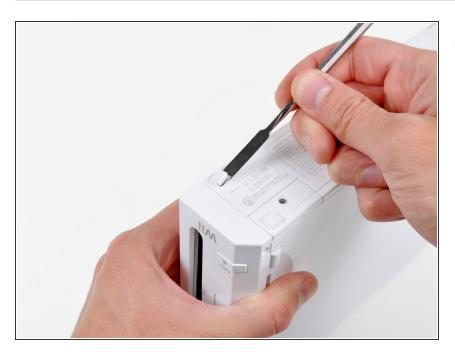
Use a metal spudger to remove the rubber foot stuck to the side of the Wii near the DVD drive opening.
