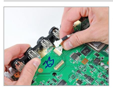
Carefully pull the DVD drive power cable away from its socket on the motherboard and remove it from the Wii.
