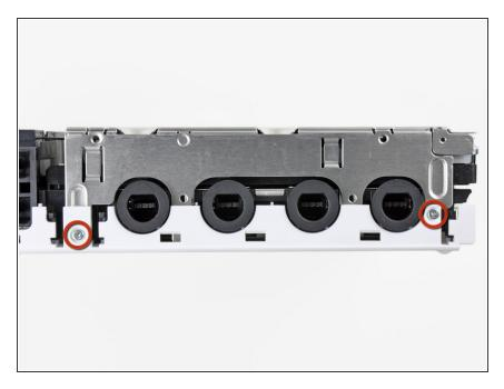
Remove the two 8.2 mm Tri-Wing screws securing the DVD drive shield near the controller ports.
