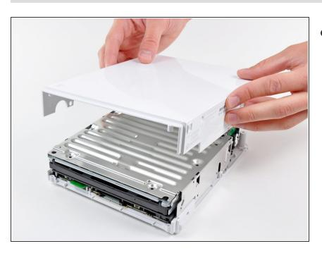
Lift the outer case straight up off the body of the Wii.
