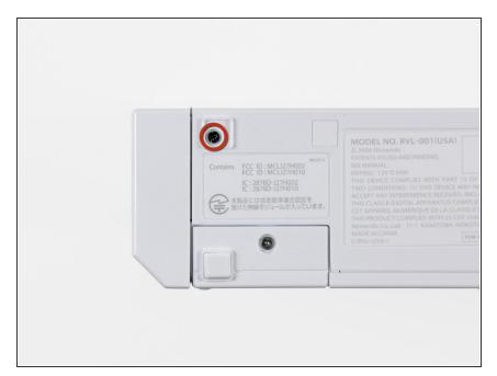
Remove the single 5.9 mm Phillips screw hidden under the foot you just removed.
