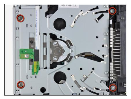
Remove the four 9 mm Phillips screws securing the DVD drive to the bottom panel.
