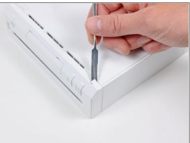
• Use a metal spudger to remove the white plastic screw covers stuck to the lower case near the front of the Wii.
