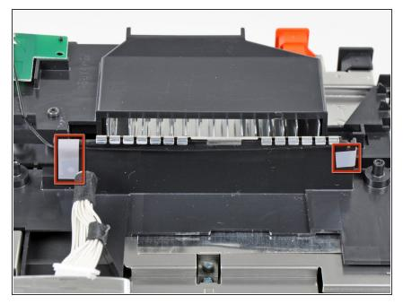
Remove the two pieces of tape securing the second Wi-Fi antenna cable to the plastic bracket near the heat sink.
