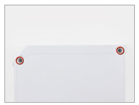
Remove the two 8.2 mm Tri-Wing screws hidden under the feet you just removed.
