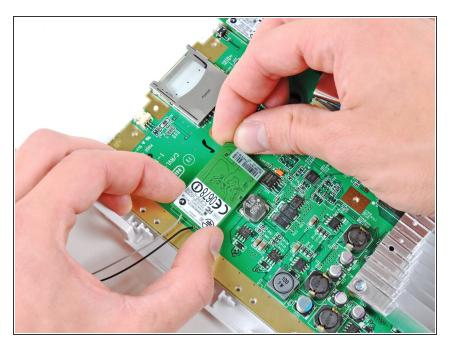
Lift the side of the Wi-Fi board furthest away from the heat sink and lift it out of its socket on the motherboard, being careful not to put too much sideways force on the connector.
