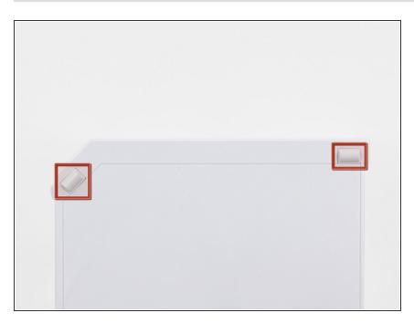
Use a metal spudger to remove the two rubber feet stuck to the bottom face of the Wii near the rear ports.
