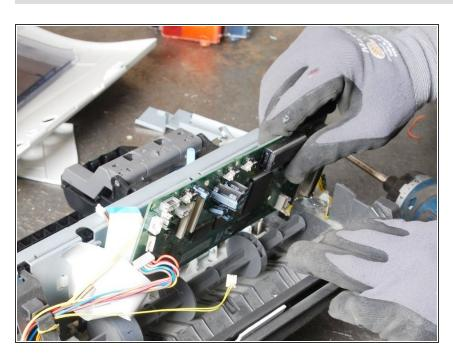
Unscrew and remove the PWB.
