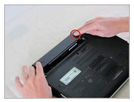
On the opposite side of the battery, press the release latch and slide the battery away from the main body to remove.
