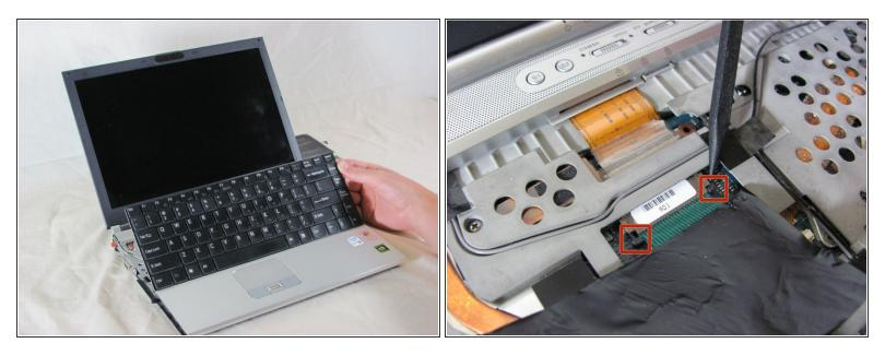
The keyboard is still attached by ribbon cable, don't try to remove the keyboard entirely yet.
