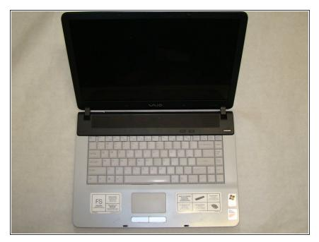
After the screws are removed, flip the laptop over so the keyboard is facing up and move the screen to its upright position.
