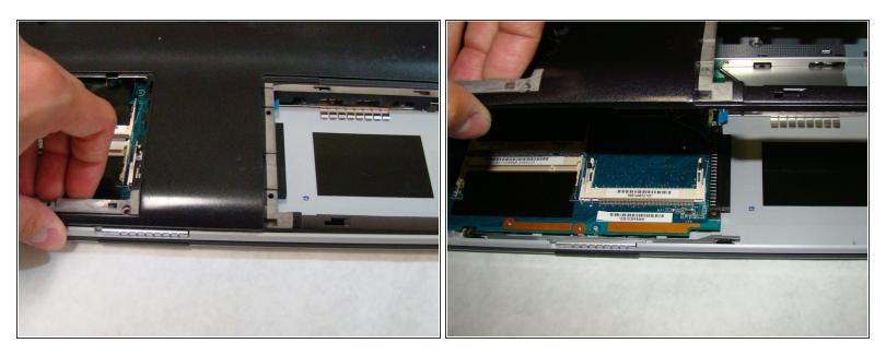
• After removing the screws, use your fingers to lift the back cover off the laptop.
