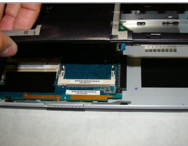
After removing the screws, use your fingers to lift the back cover off the laptop.
