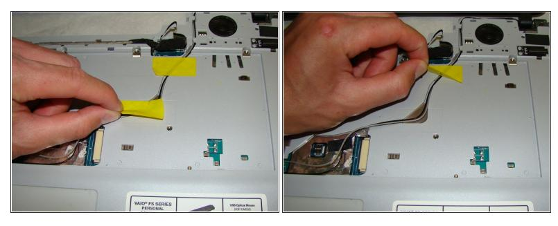
Remove the two pieces of tape that hold the display cables in their slot.
