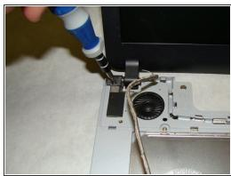
• Use a Phillips #0 screwdriver to remove the two screws (Length: 6.9 mm) that attach the screen to the body of the laptop.
