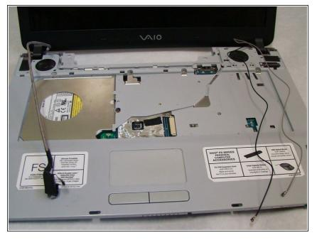
Pull the power and display cables out of their respective grooves in the body of the laptop so that they are
