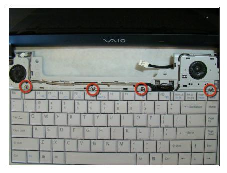
After removing the speaker cover, remove the four screws (Length: 3.6 mm) with your Phillips #0 screwdriver that hold the keyboard in place.
