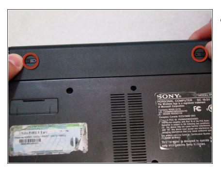
Push both latches towards the center of the battery.
