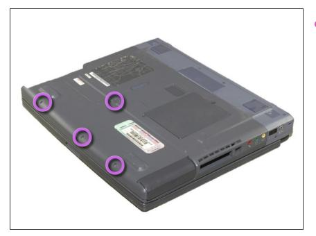
Remove the four 16mm Phillips screws bordering the edge of the laptop, indicated here.
