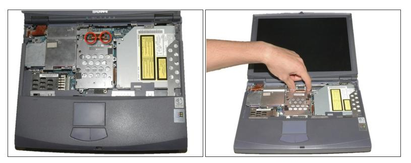
Remove the two 4mm Phillips screws in the center of the computer located on each side of the copper electrical strip.
