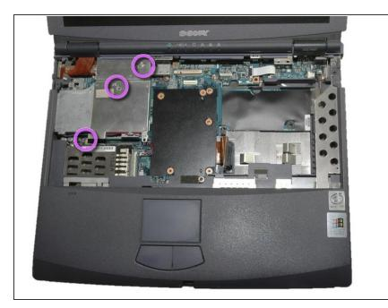
Remove the three 6mm brass colored, Phillips screws that hold the fan cage in place.
