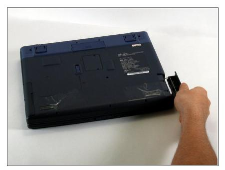
• Lift the panel up and then out to gain access to the battery.
