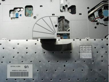
Lift up lever underneath the ribbon to detach the keyboard.
