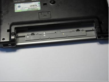
With the tabs still in the unlock position, slide the battery away from the main case.
