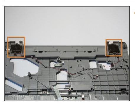
After removing the Uppercasing, flip it over and locate the two black speakers
