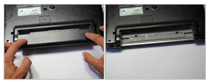
• With the tabs still in the unlock position, slide the battery away from the main case.
