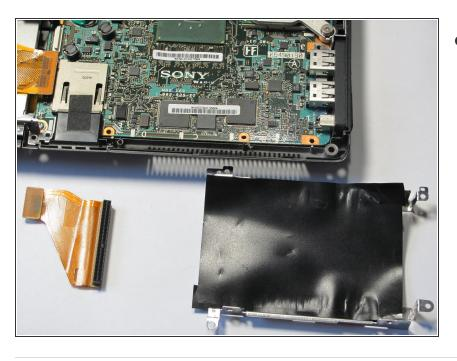
Remove the casing and the orange ribbon
