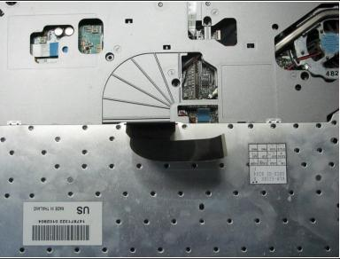
Lift up lever underneath the ribbon to detach the keyboard.
