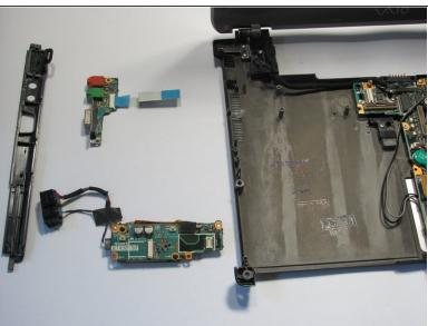
Remove the ethernet ports
