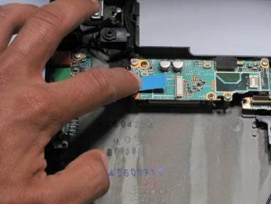
Remove the blue ribbon from the Ethernet Circuit Board
