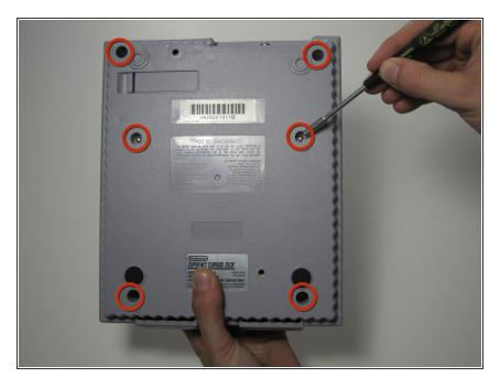
Remove the six screws located on the underside of the system using the Gamebit 4.5mm screwdriver.
