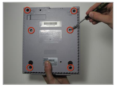
• Remove the six screws located on the underside of the system using the Gamebit 4.5mm screwdriver.
