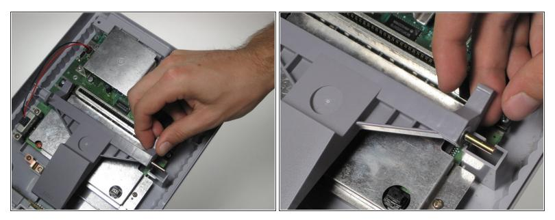
• Lift the right side of the eject lever out of the housing.
