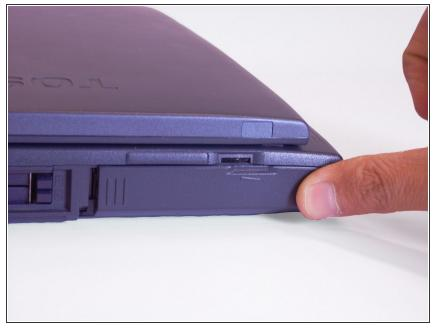
• Placing your finger on the raised grip, push the battery casing to the right. It will slide over.
