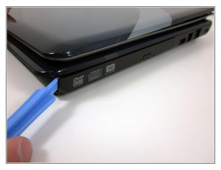
• Use the plastic opening tool to pry the CD/DVD drive out of the frame.
