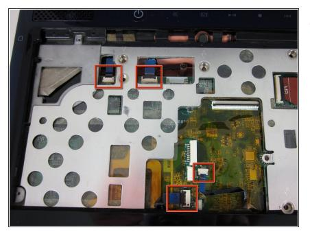
Detach the four blue ribbon cables carefully with tweezers. Some of the ribbons may require a flap to be raised because it secures the ribbon in.
