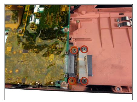
Remove these screws with a Phillips #0 screwdriver.
