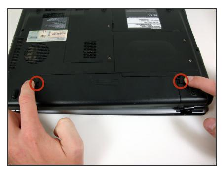
Unlatch the battery by pushing outward on both latches.
