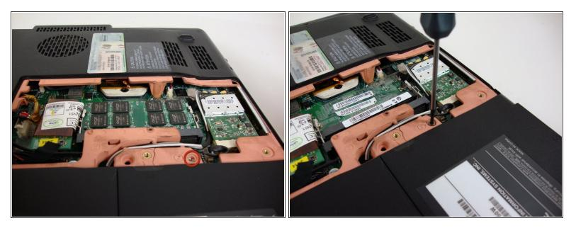
Locate and remove the circled screw with a Phillips #0 screwdriver.
