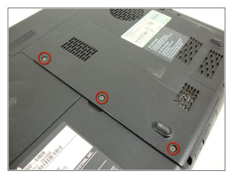
Remove the back panel by removing the three labeled screws with a Phillips #0 screwdriver.
