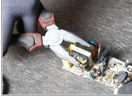
Remove all components like cooling fan, PWB, capacitors, copper coils by cutting off cables and wires and place them aside.
