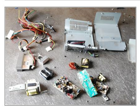
Separate the remaining materials according to their type and go on with the appropriate data sheet (e.g. aluminium, ferrous metals, cables, plastic, further PWBs, capacitors etc.).
