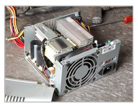
Remove the steel casing, clean it and put it aside.
