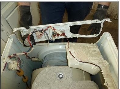
Unscrew and remove the switchboard.
