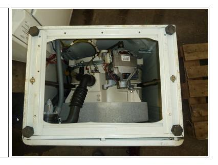
• Turn the machine upside down and open the bottom panel (if there is one).
