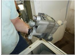
Unscrew the motor from the outside and the inside; then, remove it.
