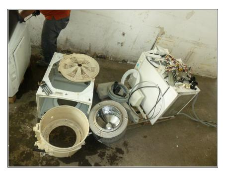
Separate the remaining materials according to their type and go on with the appropriate data sheet (e.g.
