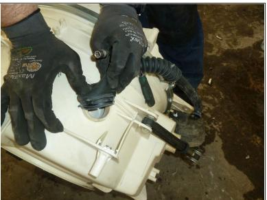
Unscrew and remove the water hose.
