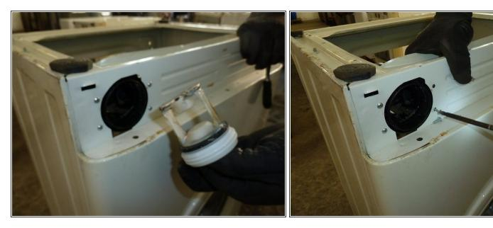
Remove the lint collector and unscrew its fixture.
