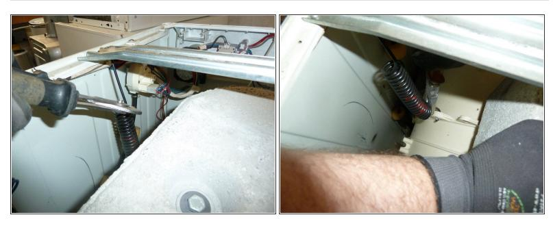
Remove the remaining springs that hold the drum.
