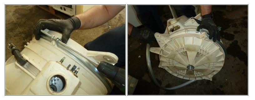
Unscrew and remove the metal belt around the plastic fixture around the drum.
