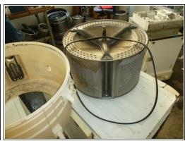
Open and remove the case around the drum.
