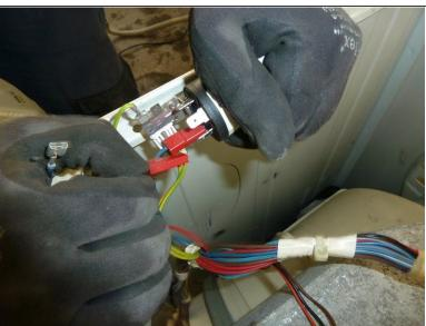
Remove the capacitor and unclip all wires, being careful not to touch the terminals as this could lead to a potentially dangerous electrical discharge.
