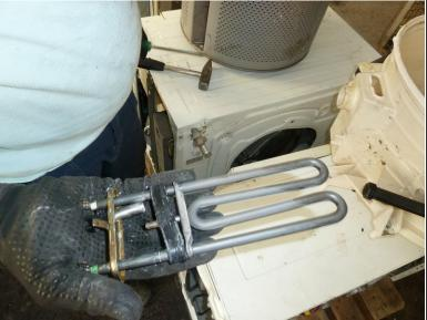
Unscrew and remove the heating element.
