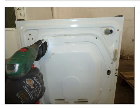
Remove the rear cover by unscrewing it.
