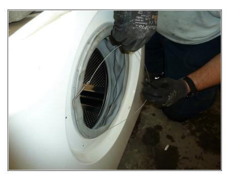
Remove the slim spring around the door opening. (It holds the rubber sealing in place).
