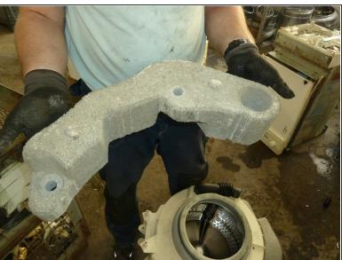
Remove the concrete weight.
