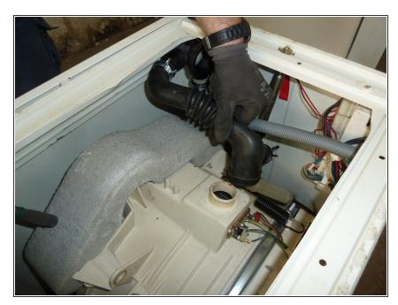
• Unplug and remove the water pipe.
