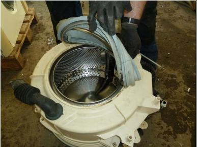
Again, remove the spring around the drum, and the rubber sealing.
