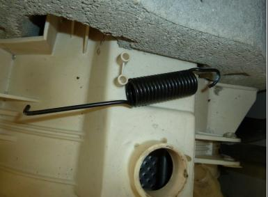
Cut and remove the springs holding the drum.
