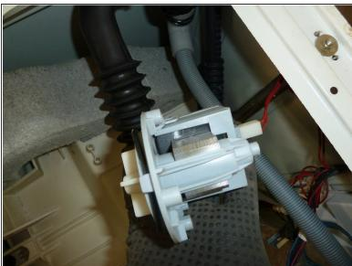
Unscrew and remove the water pump.
