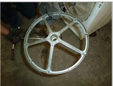
Unscrew and remove the aluminium drive wheel.
