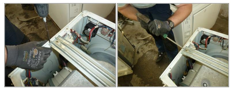
Unscrew and remove the metal bar.
