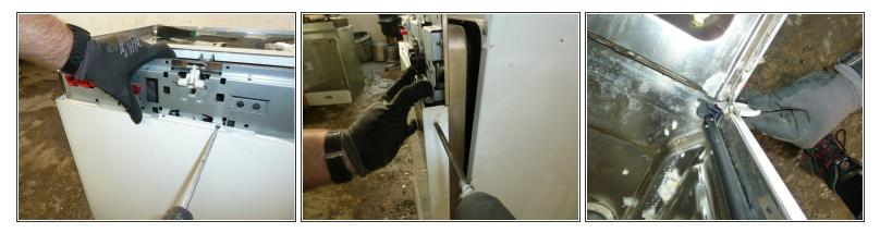
Unscrew the remaining front door panel from the outside. Remove any plastic parts protecting the door hinges.
