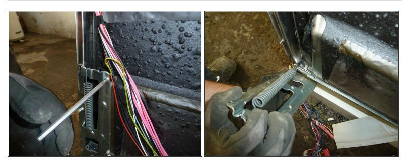
Unscrew the door hinges. Remove the hinges with the springs.
