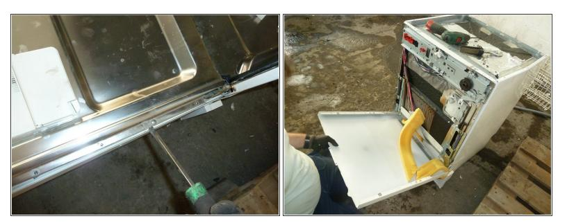
Pry off the internal stainless steel sheet. Remove the front sheet and any insulating materials.
