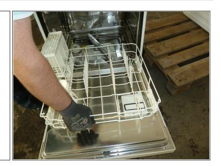
Open the front door and remove the lower dish tray.
