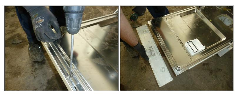
Unscrew the stainless steel interior door panel. Remove the front panel.
