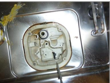
Pull out the fixture. Unscrew the next fixture parts.
