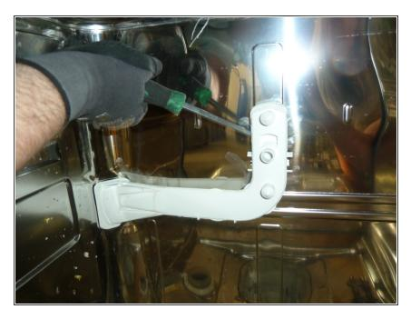
Remove plastic parts such as the injection nozzle with a large screwdriver.
