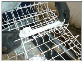
• Remove the upper dish tray. Unscrew the water dispenser. Unclip the plastic fixture.
