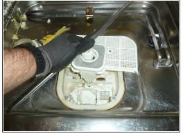
Remove plastic filters. Unscrew further filter parts. Remove the water dispenser arm. Pull out the fixture.
