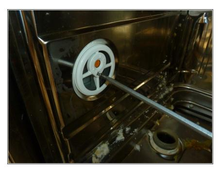
Unscrew and remove any remaining plastic parts in the interior e.g. the valve cover.
