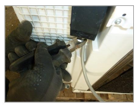
Cut off the power supply cable, dispose of the plug separately (mixed waste).
