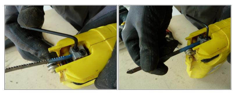
Unscrew and remove the saw blade.
