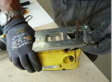
Unscrew and remove the bearing surface.
