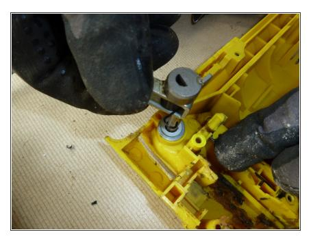
Remove the pendulum stroke.
