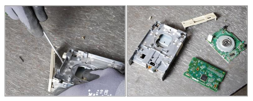
Separate the remaining materials and components, amongst others the back cover, the motor, the floppy disk reader, the metal frame, etc. Assign them to the correct material fraction (e.g. aluminium, copper, ferrous metals, plastic, further PWBs, etc.).
