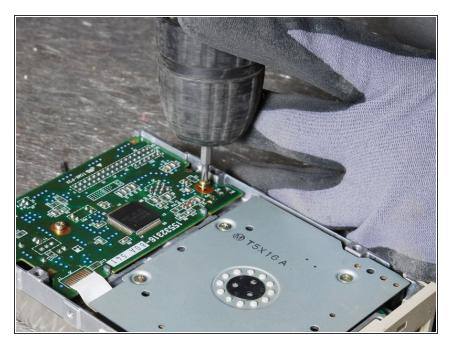
• Unscrew the PWB cover and unscrew/remove the main PWB.
