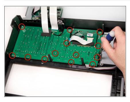
Using a Phillips #2 screwdriver, remove the thirteen 9.8 mm silver screws holding the mother board to the face plate.
