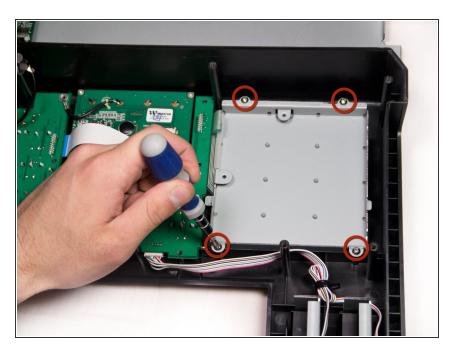
Using a Phillips #2 screwdriver, remove the four 9.8mm screws holding in the base of the beat pad.
