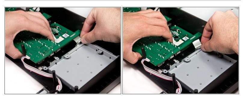
Slightly lift the mother board near the edge of the beat pads and wiggle the beat pad ribbon connector free.
