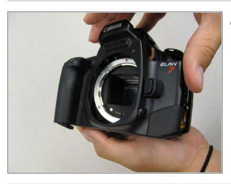
Remove the front panel by lifting out the side opposite the grip.
