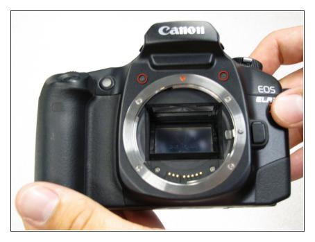
Remove two 4.8 mm black screws on the front of the camera.
