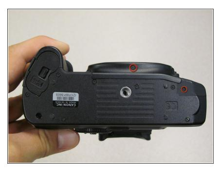
Remove one 4.3 mm black screw under the lens ring and one 4.8 mm black screw on the bottom of the camera.
